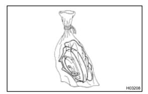
(i) Dispose of the steering wheel pad (with airbag). **CAUTION:**
