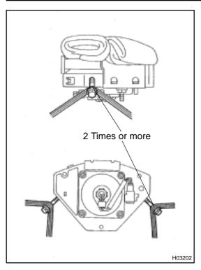
Using 3 wire harness, wind the wire harness at least2 times each around the bolts installed on the leftand right sides of the steering wheel pad.
